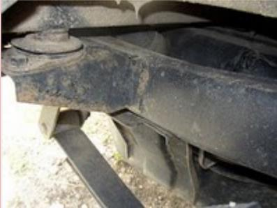
Since frames are made of steel they will rust, and usually from the inside out. But what you may have noticed on older 4WDs is that the frame rarely rusts near the engine compartment. Many people think this is due to heat generated by the engine which keeps things drier and therefore less prone to rust.
